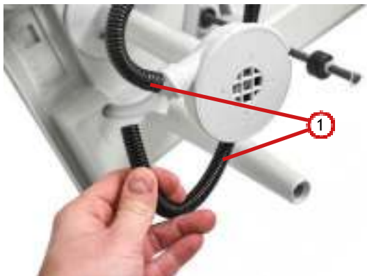
Fig. 6.3.4.4: Pulling off the pump hoses
