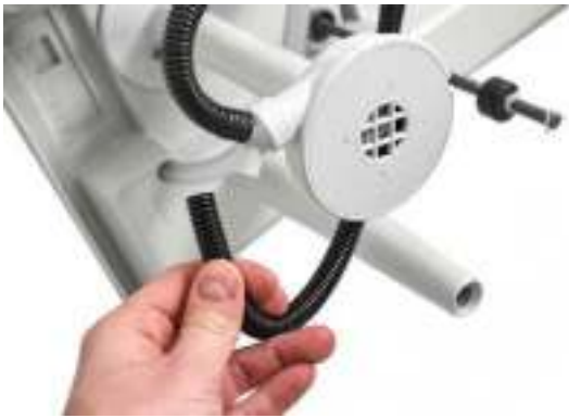
Fig. 7.4.1.5: Pulling off the pump hoses
