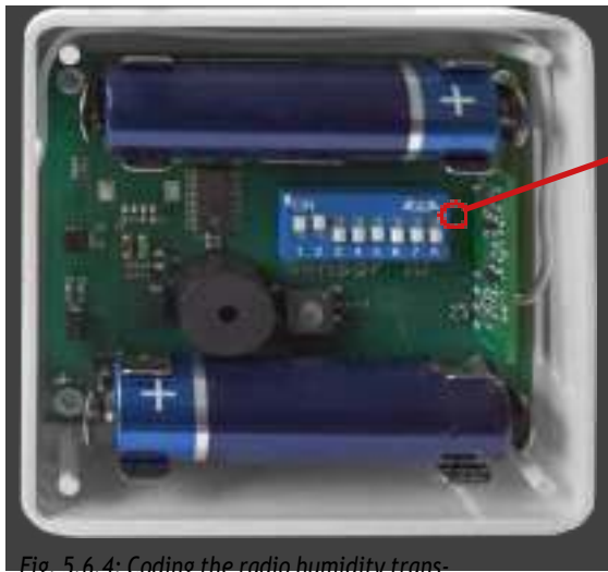
Fig. 5.6.4: Coding the radio humidity transmitter
