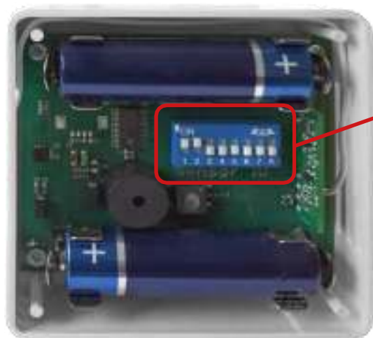
Fig. 5.6.1: Interior view of radio humidity transmitter
