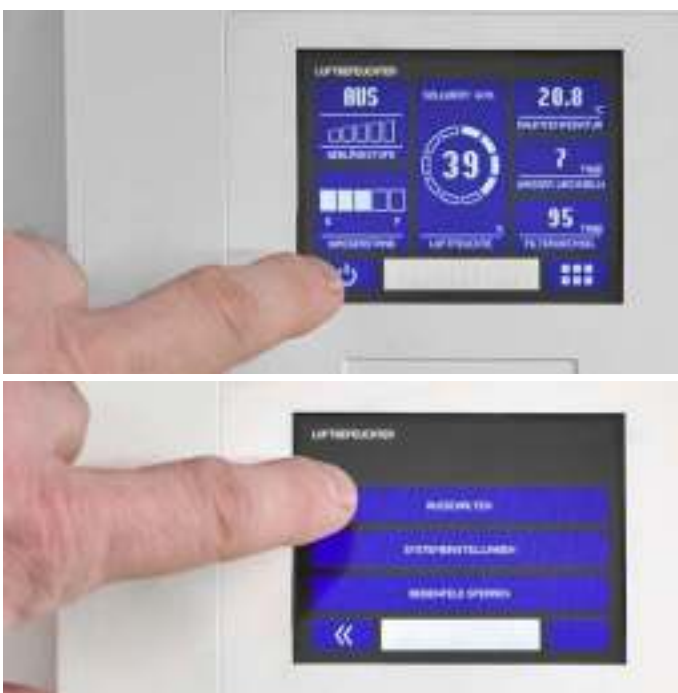
Fig. 5.2.2: Switching off the unit
