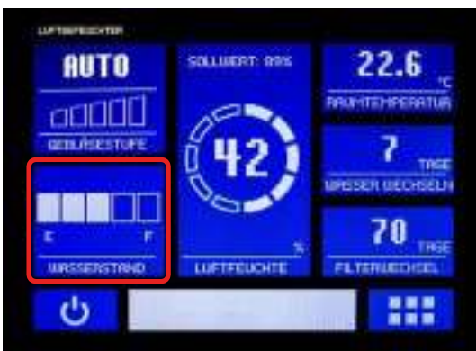
Fig. 5.1.2: Water level display
